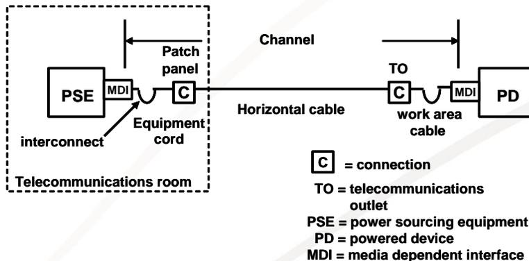
Figure 9. Powered Interconnect Configuration
