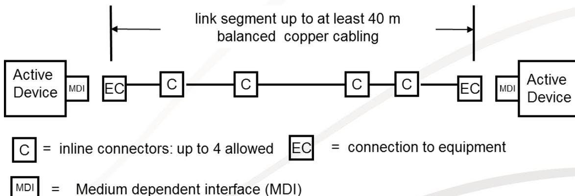
Figure 4. Example 1000BASE-T1 Link Segment type B
