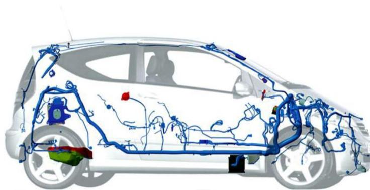
Figure 2. Automotive wiring system example
