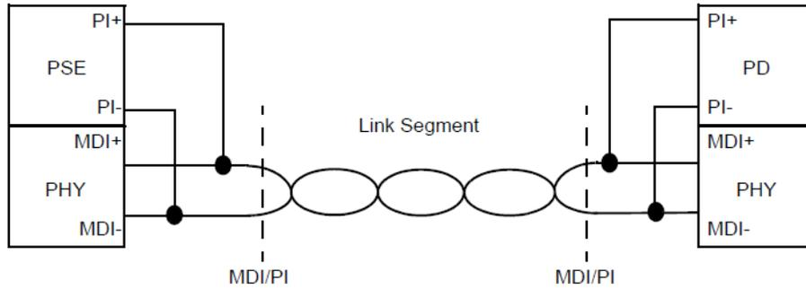
Figure 8. PoDL system block diagram
