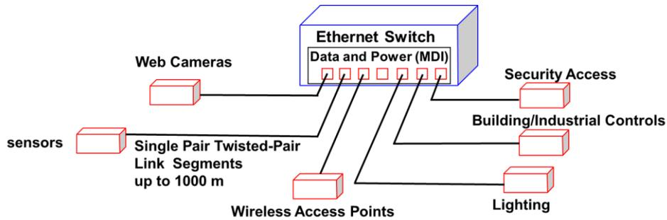
Figure 1. 802.3cg single pair Ethernet 10 Mb/s and power
