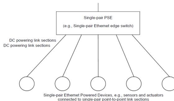
Figure 6. Point-to-point powering topology
