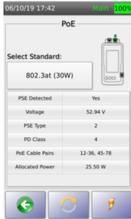
Example Cat6A PoE Test Results
