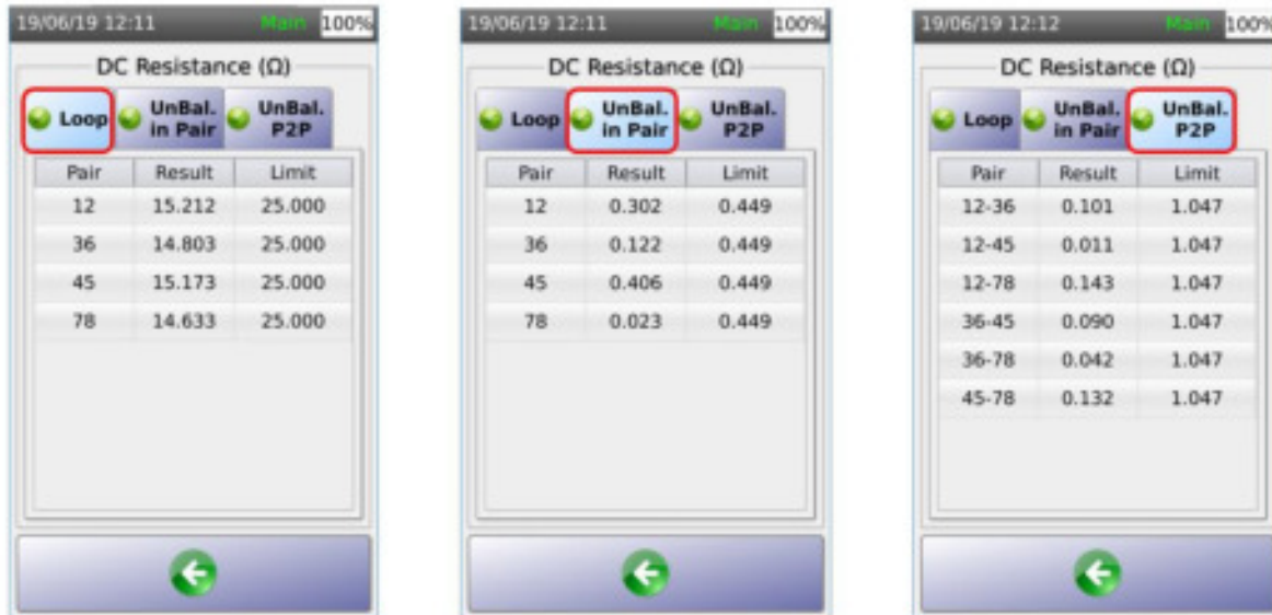
Figure 6: Resistance and Resistance Unbalance Measurement
