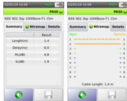
Fig 16 : Single Pair Ethernet (SPE) cable integrity assurance
