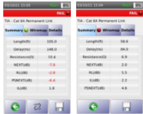
Fig 15 : Four Pair Ethernet cable integrity assurance
