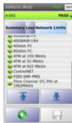
Fig 13 : Based on the performance of the cable tested, it is useful to be able to have a detailed view on what network types the link is capable of supporting
