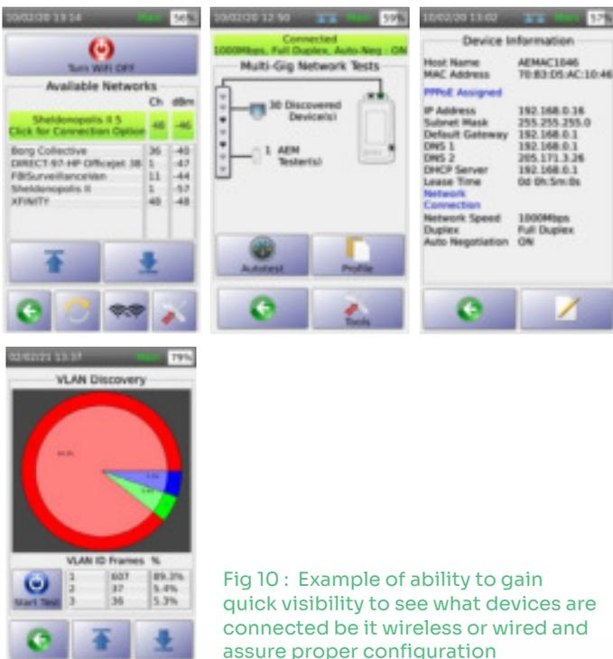
Fig 10 : Example of ability to gain quick visibility to see what devices are connected be it wireless or wired and assure proper configuration
