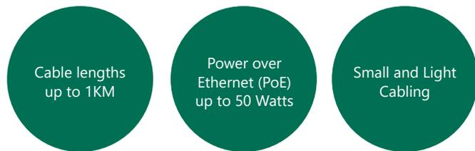
For these reasons, SPE can be an ideal choice for IoT projects that require hundreds or thousands of sensors to be placed across a campus. The small and light cable footprint with the ability to run very long runs with power delivery is quite impressive and useful in many situations.
