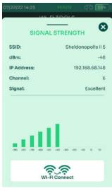
Useful for moves/adds/changes as well as general troubleshooting, TestPro will connect to a live network through the AD-NETCABLE adapter, or wireless using the optional Edimax Wi-Fi USB adapter.
