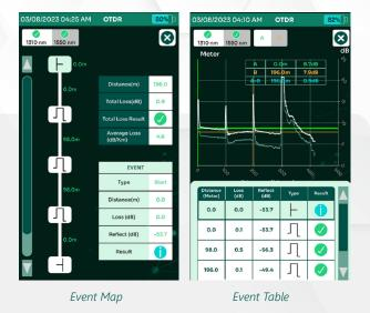
**Printed Reports:** At the completion of a test, you have the option to save the test result to memory for later upload into the included TestDataPro results management database.
